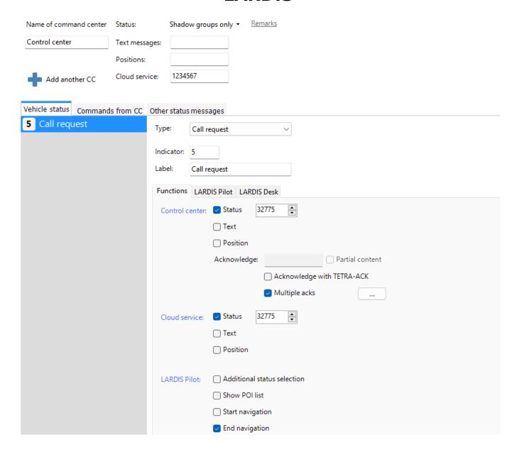
The instructions sent by the control station (usually Flash-SDS / PID 137) can be defined specifically and configured with further actions.
